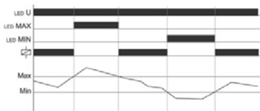
When the supply voltage  $U$  is applied, the output relay  $R$  switches into on-position, if the measured voltage is within the adjusted window. When the measured voltage left the window between MIN and MAX, the output relay  $R$  switches into off-position. The output relay  $R$  switches into on-position again, if the voltage re-enter the adjusted window.
