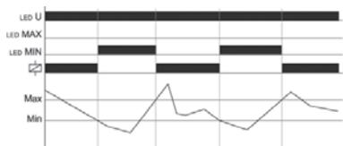
When the supply voltage  $U$  is applied, the output relay  $R$  switches into on-position, if the measured voltage is beyond the MIN-value. When the measured voltage falls below the MIN-value, the output relay  $R$  switches into off-position. The output relay  $R$  switches into on-position again, if the voltage exceeds the MAX-value.
